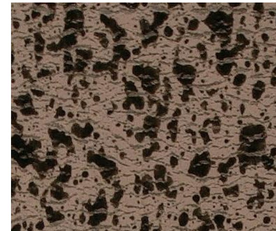
Paint cracking and debonding at a small scale
